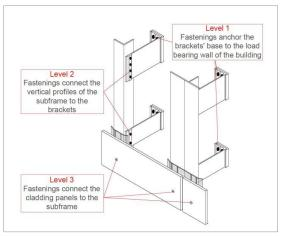
IMAGE 3 - THE DIAGRAM SHOWS THE 3 FIXING LEVELS USED AS A CONVENTION IN THIS DOCUMENT
