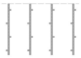
IMAGE 6 – IT IS GOOD PRACTICE TO ARRANGE THE BRACKETS OF EACH BATTEN/PROFILE ALTERNATELY
