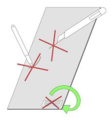
IMAGE 44 – PARTICULAR CARE MUST BE TAKEN NOT TO DAMAGE THE VISIBLE SURFACE OF THE PANELS DURING WORK ON SITE
