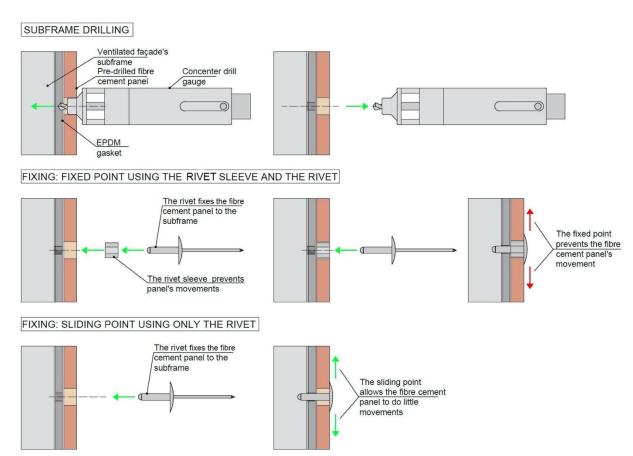
IMAGE 21 – EXAMPLE OF STEPS TO FIX KØL FIBRE CEMENT PANELS. THE PANELS ARE PRE-DRILLED WITH HOLES THAT ALL HAVE THE SAME DIAMETER OF 9.5 MM (3/8"). THE EXAMPLE SHOWS HOW THE DIAMETERS OF THE HOLES FOR THE FIXED POINTS ARE REDUCED USING SUITABLE METAL BUSHINGS.
