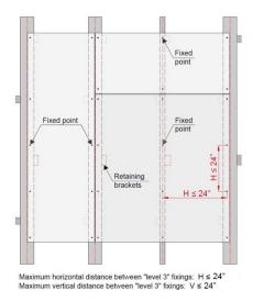
IMAGE 18 – EXAMPLE OF CLADDING WITH KØL FIBRE CEMENT PANELS. THE RETAINING BRACKET SHOWN IN RED SHOULD BE AS CLOSE AS POSSIBLE TO THE FIXED POINT OF THE PANEL.
