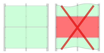
IMAGE 23 – LEFT: EXAMPLE OF A CORRECT WAY TO SECURE KØL PANELS, WITH THE HORIZONTAL JOINT OF THE CLADDING ALIGNING WITH THE EXPANSION JOINT OF THE SUBFRAME PROFILES. RIGHT: EXAMPLE OF AN INCORRECT WAY TO SECURE THE KØL PANELS, WITH A CLADDING SHEET SECURED TO TWO PROFILES.
