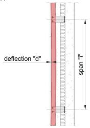
IMAGE 7 – THE MAXIMUM DEFLECTION OF THE BATTENS/PROFILES BETWEEN TWO BRACKETS DMAX MUST BE  $\leq 1/200$  for the SPAN Between the Brackets "I"
