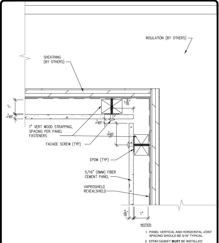
EPDM GASKET MUST BE INSTALLED CONTINUOUSLY ON ALL SUBFRAMING.
